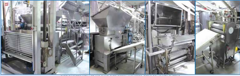
PADDLE MIXERS WITH LIFT AND DUMP, EXTRUDERS/LAMINATORS, SIZING ROLLS WITH SLITTING
