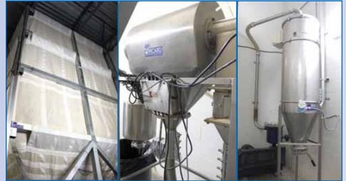
PICARD FLEXIBLE POWDER SILO WITH ROTARY SIFTER AND DUST COLLECTOR
