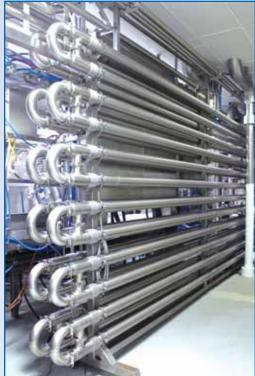
WCB 12-PASS TUBE IN TUBE PASTEURIZER
