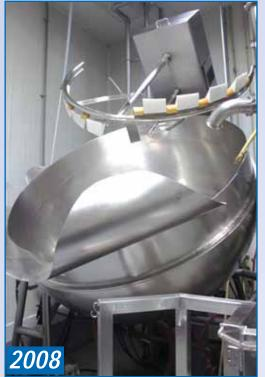
ESCAN 400 GALLON COOK/COOL TWIN AGITATED SWEEP SCRAPE TILT POUR KETTLE WITH CENTER BOTTOM OUTLET
