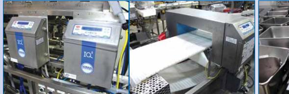
LATE MODEL LOMA IQ2 PIPELINE AND CONVEYORIZED METAL DETECTORS
